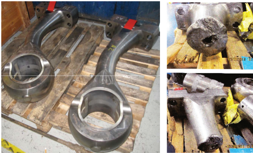
FIGURE 1. PICTURES OF THE FAILED CONNECTING RODS
